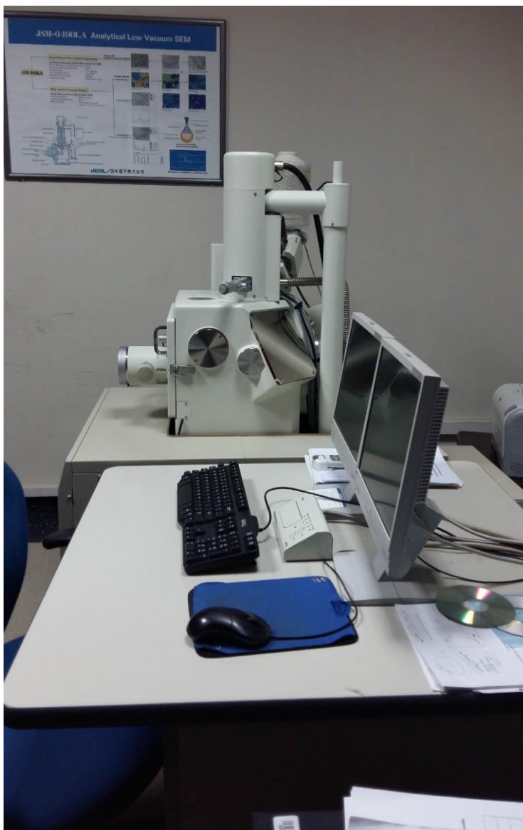
Fig. 1. Scanning Electron Microscope (JSM 6490LA) Equipped with EDS Analyzer (Courtesy: School of Chemical & Materials Engineering (SCME), National University of Sciences and Technology (NUST), Islamabad, Pakistan.)
