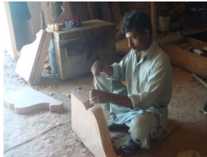
Fig. 9 - Sandstone brackets (original design).
